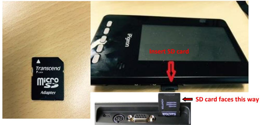
To update the iPigeon firmware is easy by using an SD memory card. Normally the iPigeon firmware is around 1 megabyte and is compressed in a zip file. You just unzip the file contents which you then copy and paste into the SD card root directory.
