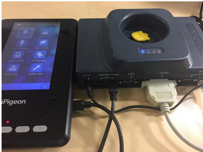
This is Mini Din which provides power and signal between Club Antenna and Clock. If the cable is not fully insert into the connector it will cause power unstable.
